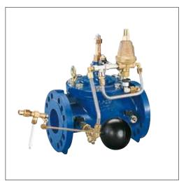
• It prevents from overflowing and maintains a constant level in the tank thanks to a float and guarantees a minimum upstream pressure.
