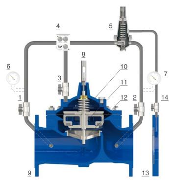
The CSA model XLC 330/430 is operated by a two 2 ways pilot (5), for flow control, with pre-set set and adjustable values, sensing the drop in pressure produced by the orifice plate (13), where a stainless steel disk is inserted inside a flange and connected to the pilot with a sensing line (14) non supplied.
